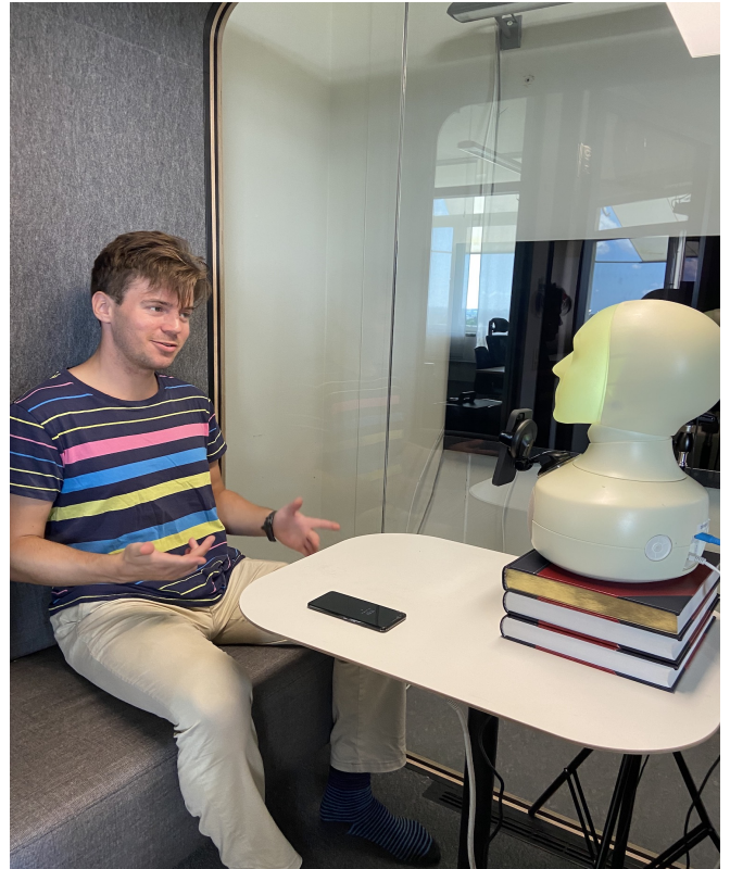
Fig. 2. The participants were interacting with the Furhat robot in a soundproof booth. On the table there was also a phone for rating the objects during the interaction.
